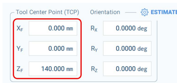
Fig. 6-12: Tool Center Point
