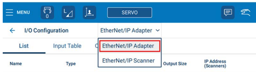
Fig. 7-33: Selecting EtherNet/IP Adapter
