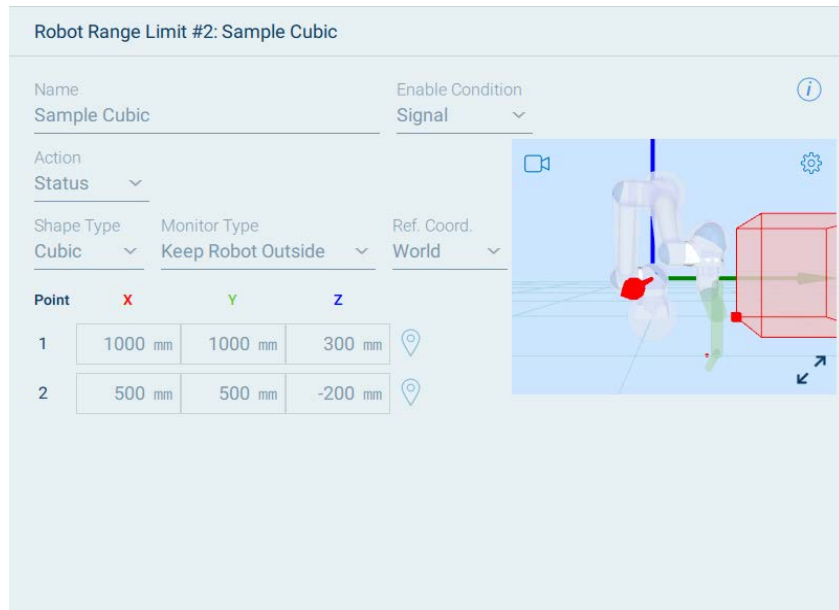
Fig. 12-8: 3D Viewer Inside Safety Settings Detail Panel
